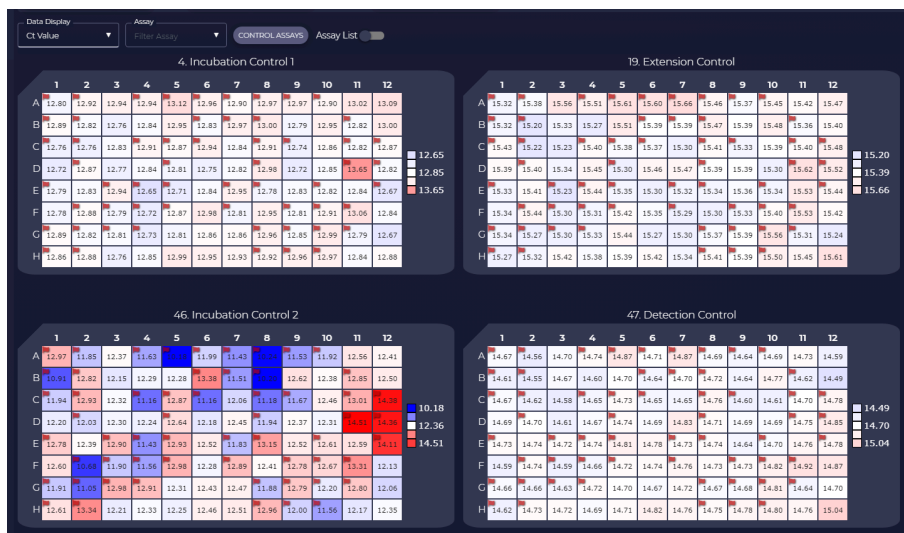
Figure 9. Ct values that show primer contamination of Incubation Control 2.
