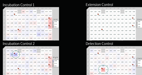
Figure 2. Data analysis example of deviating internal controls. The circled sample to the left has a deviating Incubation Control. The circled sample to the right has deviating Detection Control and Extension Control.
